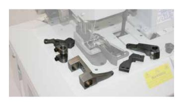
One of the salient features of our net sewing machine BURASCHI RP7 BR PNEUMATIC is that the key components are specially made from solid of the AISI 315 special alloy, extremely superior to the casted components of the traditional machines. In addition, our key components, heat treated with differentiated application in the critical area, are extremely strong, durable and reliable.
