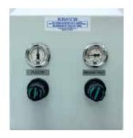
Inside the box above it was possible to achieve and to concentrate with the utmost care all the pneumatic and electro-pneumatic commands of our machine. Therefore, the maintenance, the control and the setting are somewhat facilitated.
