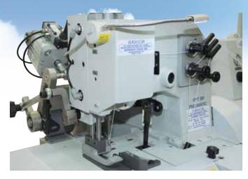
Detail of the net sewing machine RP7 BR PNEUMATIC, showing the operational area and many key components made from solid of the AISI 315 special alloy.
